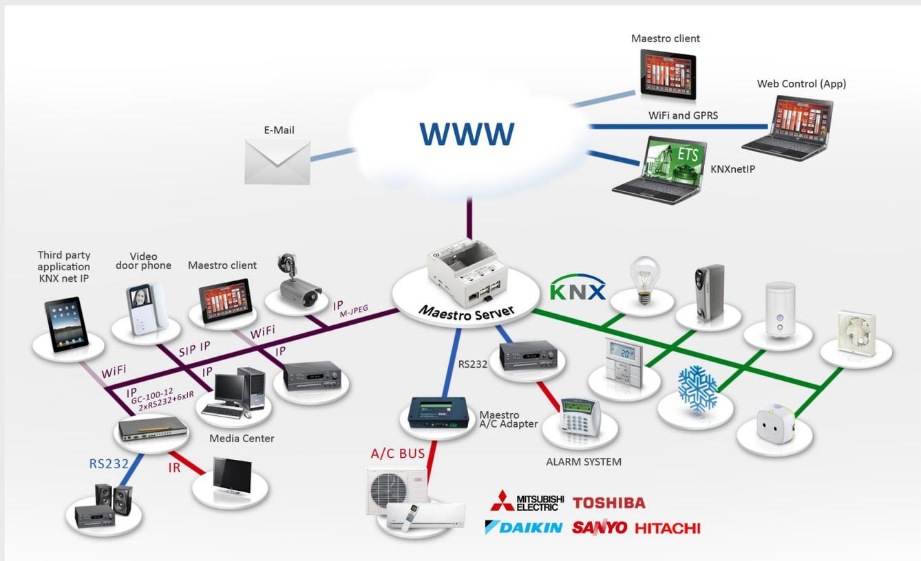
Maestro is KNXnet/IP-enabled so technicians can program and monitor KNX devices remotely via the Ethernet/internet, without any need to travel to the location
